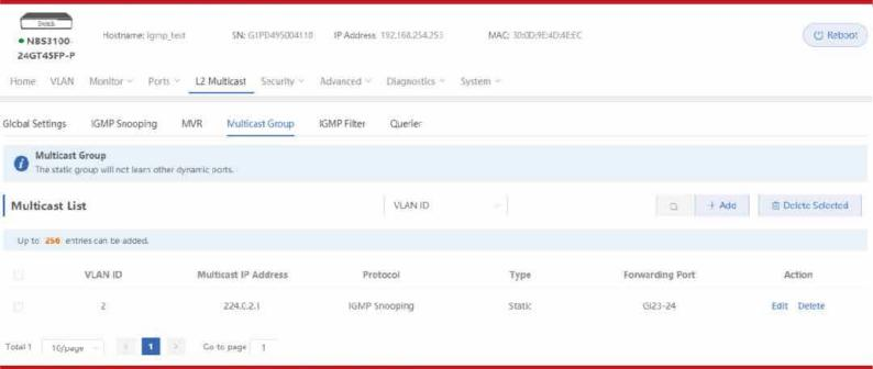
5. L2 Multicast > IGMP Filter Define Profile ID, multicast IP range that will be allowed and choose behaviour permit to allow it. apply filter on switch port that connected to end user devices.
